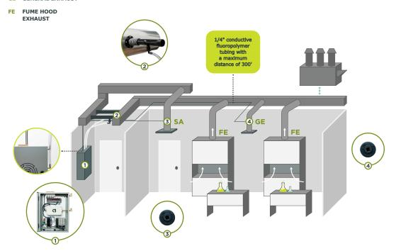
Reducing ventilation in laboratories and vivariums based on real-time sensing offers opportunities for energy conservation. This approach can safely reduce lab air change rates to as low as two ACH when the lab air is "clean" and the fume hood exhaust or room cooling load requirements do not require higher airflow rates. Research by Sharp (2010) showed that lab rooms are on average "clean" of contaminants in excess of about 98% of the time.
