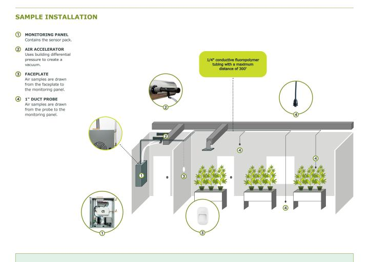
AntrumX provides **more sensing with fewer sensors**, and locates the sensor pack outside of the environment so the grow rooms are wash-down ready.
