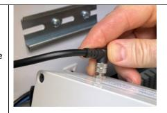
Position the spring-loaded lower lip of the DIN rail mount on the back of the sensor pack under the lower edge of the DIN rail.
