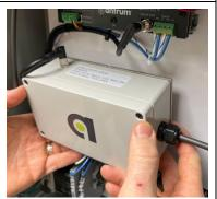
Slide the sensor pack to the right while positioning the 1/4" tubing to align with the bulkhead fitting(s). Using gentle pressure, insert the ¼" tubing into the fitting(s).
