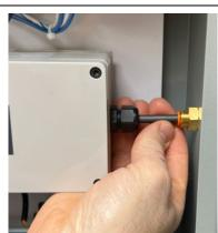
Maneuver the ¼" tube extending down from the manifold to align with the elbow push-toconnect fitting on the sensor pack. Gently Insert the tubing into the fitting.
