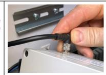
Position the spring-loaded lower lip of the DIN rail mount on the back of the sensor pack under the lower edge of the DIN rail.
