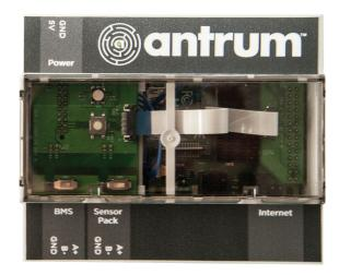
The core of the AntrumX<sup>™</sup> technology platform is the gateway, a controller located in the monitoring panel that integrates the sensor pack, building management system (BMS), and the cloud.
